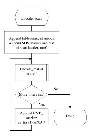
Figure D.3: Control procedure for encoding a scan
