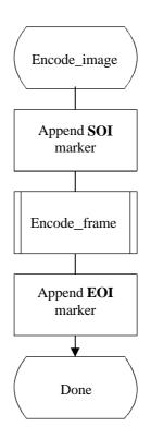
Figure D.1: Control procedure for encoding an image
