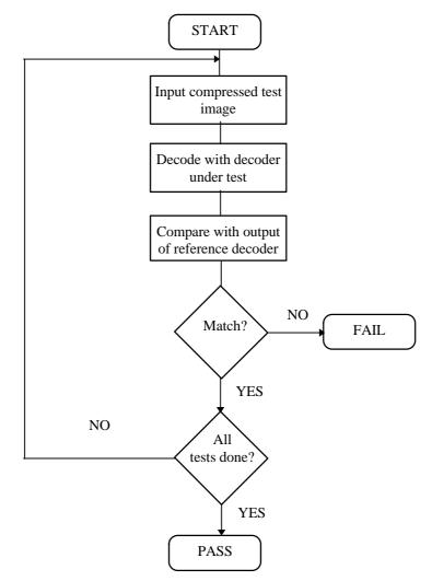
**Figure 6: Decoder testing procedure**
