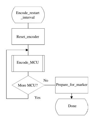
Figure D.4: Control procedure for encoding a restart interval
