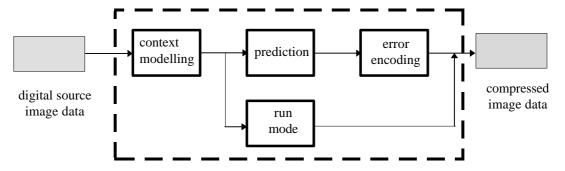
Figure1 : Lossless encoder simplified diagram
