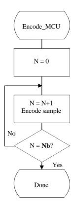
Figure D.5: Control procedure for encoding a minimum coded unit (MCU)
