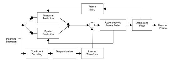
Figure 4.1: Block diagram of the RealVideo 8 decoder algorithm
