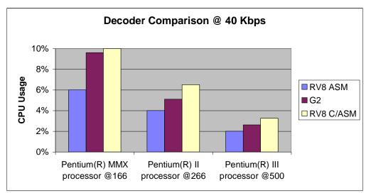
RV8 C/ASM is an estimate for a RV8 decoder using C for everything except the postfilter.
