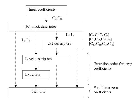
The main code object, 4x4 block descriptor is transmitted first. Based on the values of its components, subsequent code objects: 2x2 descriptors, level descriptors, and sign bits may follow.
