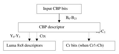
The main CBP object, CBP descriptor is transmitted first using one of the canonic Huffman codes (see Section 5.4.6) corresponding to the current macro-block type, and quantizer step size.
