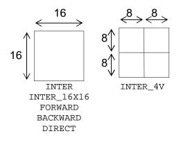
Figure 4.5: Motion compensation block sizes for Inter macroblocks
